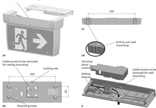
Figure 1: Mounting holes position for wall or ceiling mount Figure 2: Terminal block connection and internal view
